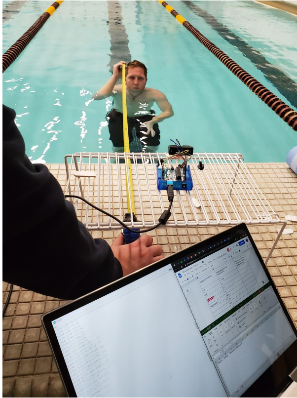
Figure 6: Image testing the IR sensor
